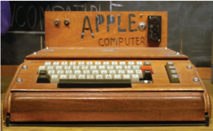
FIG 3 The original Apple I computer built by Steve Wozniak. (Image courtesy of Wikipedia.)
