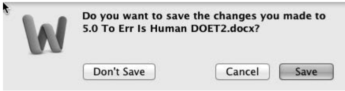
FIGURE 4.6 A Lock-In Forcing Function. This lock-in makes it difficult to exit a program without either saving the work or consciously saying not to. Notice that it is politely configured so that the desired operation can be taken right from the message.
