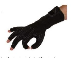
A first approach to integrate electronics into textile structures was certainly achieved by gloves wired to the computer that allows it to take input from user's hand gestures. Sensors in the glove detect (Figure 11) the wearer's hand movements. Four wires were used for each finger or tube to build up a circuit. The voltages coming out are varying depending on the finger position [65].
