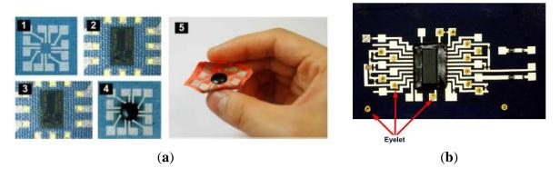
The P-FCB substrate is fabricated using woven fabrics. The planar electrodes are deposited on the fabric patch directly by silk screening of conducting epoxy or by gold sputtering. First, the circuit board is silkscreen printed on the fabric patch. Then the IC is placed on the fabric and wire-bonded to the patterned electrodes. Finally, the IC is molded with non-conductive epoxy (Figure 16a) [89].
