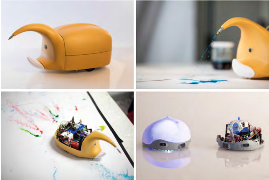
Fig. 10. Further designs for the niche constructing drawing robots, developed by Nick Jones, based on the insect species Stenaptinus insignis . These insects fire a toxic acid spray when attacked. The microphone, which responds to sounds, can be seen in the middle of the front of the robot. These robots are currently under development.
