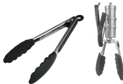
(Below) Figure 3. Repurposed kitchen tongs to claw
