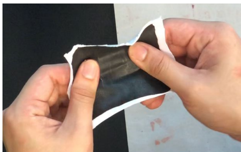
(Figure 4: Lycra Spandex losing all flexibility after LDPE fusion)
