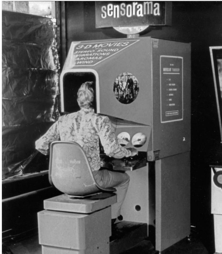
*Figure 4: Sensorama Simulator by Morton Heilig*
