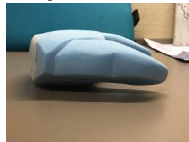
Adding epoxy and sanding the streamline of the form
