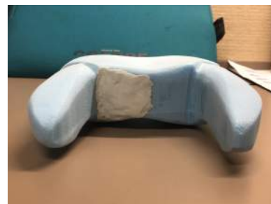
Adding epoxy and sanding the streamline of the form
